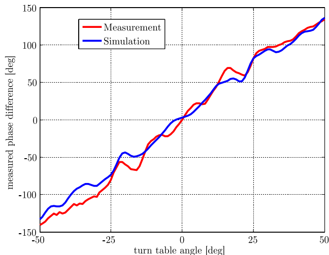
Fig. 8. Measured phase difference between the two channels for a single radar target
